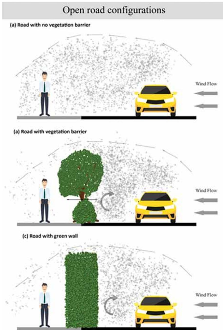
**Figure 04 –How the PM is reduced behind the green fence**
