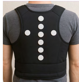
Figure 2: Vibrotactile vest, Six actuators to send phonemes through spatial binary patterns and two additional actuators to represent environmental sound attributes
